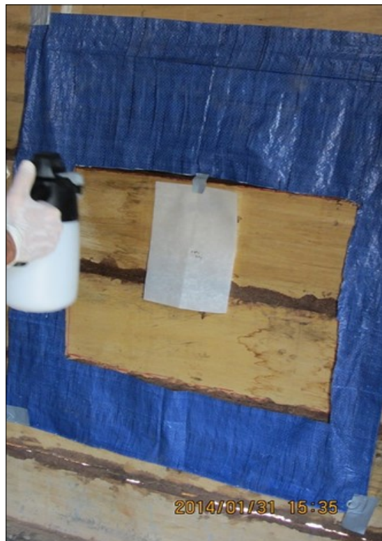
Figure 2. Applying insecticide with a flat fan, small volume sprayer on the wall field limited by a holed tarpaulin frame and with a Whatman paper attached at the middle of the spray field for collecting spray data.
